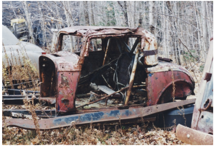
Right side view shows the door skin missing and the limited roll cage protection. (Towne photo)
